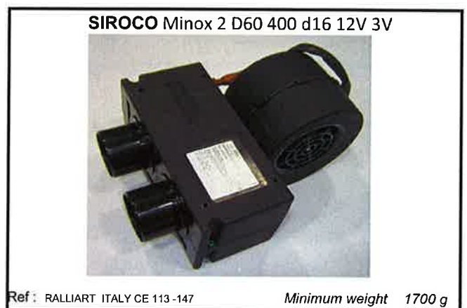
PHOTO N° 12 Heating / Demisting system
